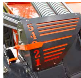
Optional hydraulic stubble height adjustment for easy setting from tractor cab.
