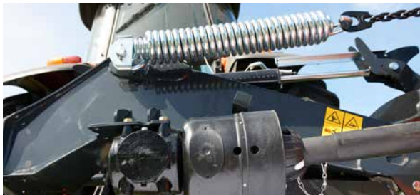
Two speed gearbox – switched by turning the main gearbox 180°.
