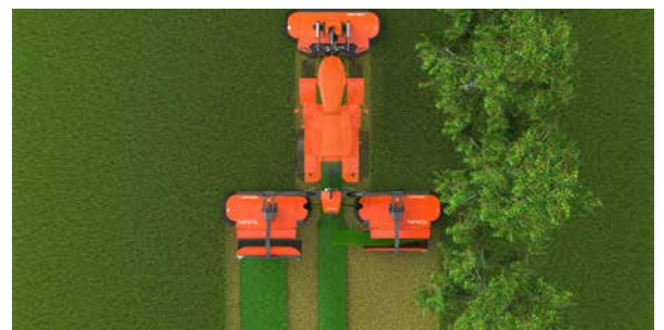
Using one belt to move crop away from field boundaries.
