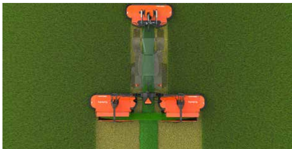
One large swath from 10m working width.
