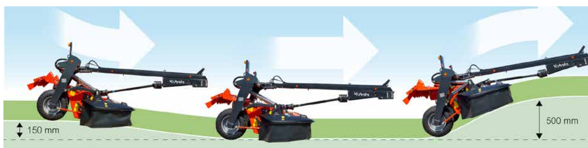
Optional hydraulic stubble height adjustment for easy setting from tractor cab.
