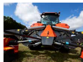
Large compensating spring ensures excellent flotation across the full mower width.
