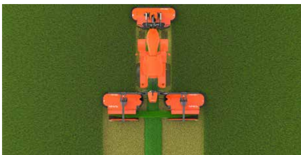
One large swath from 8.7 or 9.5m working width.
