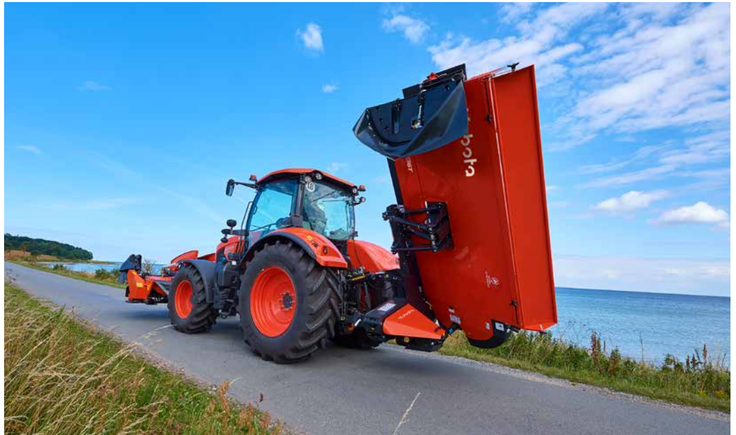
DMC6336T Vario in transport. The telescopic frame arm moves to the lowest possible position to reach a transport height of only 3.70m.
